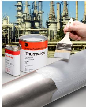
**THURMALOX 225HD** — A high build silicone primer applied to insulated and un-insulated carbon and stainless steel surfaces with a maximum heat resistance of 1200°F (649°C). Thurmalox 225HD offers high build protection for deep profile blasted surfaces. Suitable finish coats for Thurmalox 225HD include Thurmalox 230/230C and 280/280C series.
