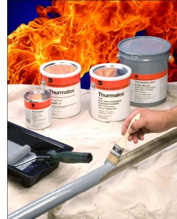
**THURMALOX 218/219** — A two component modified silicone designed for the protection of insulated carbon and stainless steel surfaces with a maximum heat resistance of 450°F (232°C) continuous with peaks to 500°F (260°C). Thurmalox 218/219 is formulated for both ambient and hot applied installations up to 300°F (177°C) and can be re-insulated in 24 hours at 77°F (25°C).
