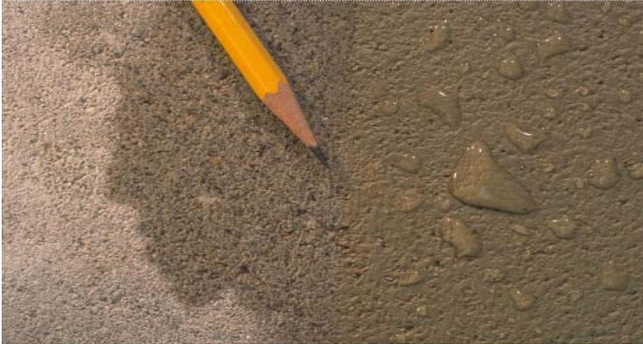
**Treating concrete with Dymacryl allows water to bead (right) while untreated concrete (left) is deeply stained by water absorption. Dymacryl prevents water penetration, thereby preserving the appearance of exposed masonry.**
