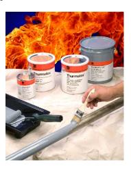
**THURMALOX 218/219** — A two component modified silicone designed for the protection of insulated carbon and stainless steel surfaces with a maximum heat resistance of 450°F (232°C) continuous with peaks to 500°F (260°C). Thurmalox 218/219 is formulated for both ambient and hot applied installations up to 300°F (177°C) and can be re-insulated in 24 hours at 77°F (25°C).
